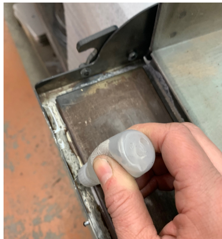
Apply gasket glue into the channel
