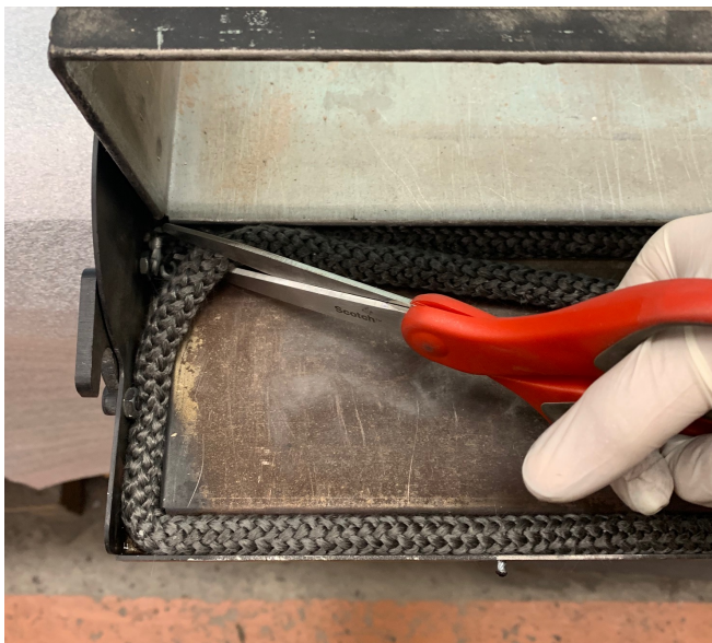
Use scissors to cut the gasket- leave enough gasket to butt the ends
