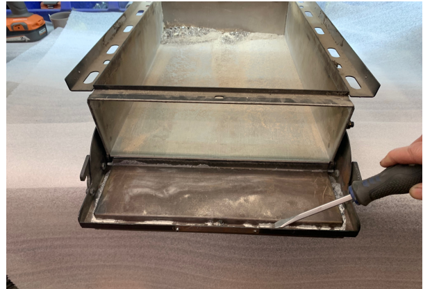
Use a screwdriver or putty knife to remove residual glue
