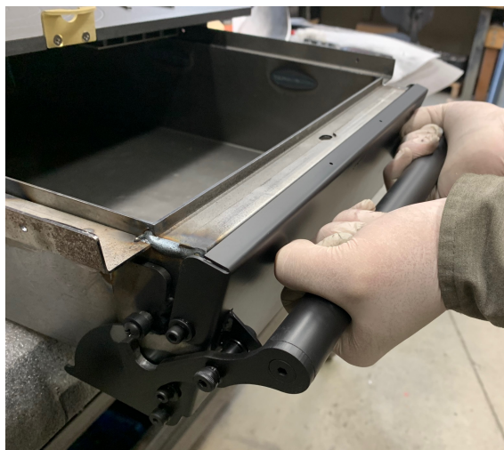
Use both hands and lift up on the handle to unlatch
